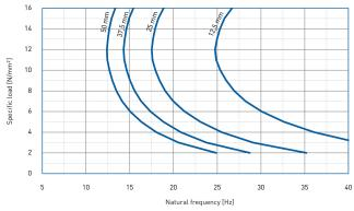
Natural frequency of a single-degree-of-freedom system consisting of a fixed mass and an elastic bearing consisting of VIKADYN VD 12000 on a stiff subgrade.
