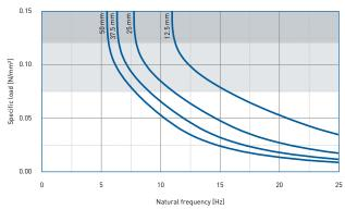
Natural frequency of a single-degree-of-freedom system consisting of a fixed mass and an elastic bearing consisting of VIKADYN VD 150 on a stiff subgrade.
