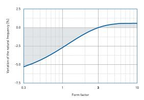
Correction values varying form factors specific load 0.15 N/mm<sup>2</sup>. Form factor q = 3
