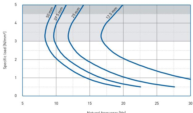
Natural frequency of a single-degree-of-freedom system consisting of a fixed mass and an elastic bearing consisting of VIKADYN VD 350 on a stiff subgrade.
