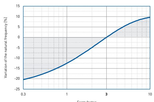
Correction values varying form factors specific load 0.35 N/mm².
