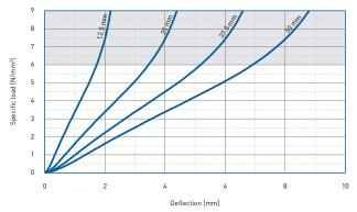
Recording of the 3rd loading; testing between steel plates at room temperature measured with a deflection rate of 1% of the thickness per second.
