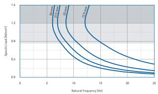
Natural frequency of a single-degree-of-freedom system consisting of a fixed mass and an elastic bearing consisting of VIKADYN VD 350 on a stiff subgrade.
