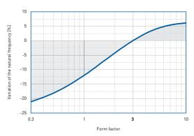
Correction values varying form factors specific load  $0.35 \text{ N/mm}^2$ . Form factor q = 3
